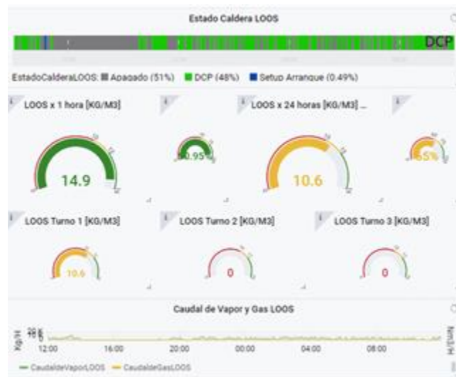
Fig.3. Dashboard that shows the status of a boiler from data gathered by the IIoT architecture. Source: Authors.
