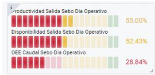
Fig. 2. KPI of the daily operation that is shown in the dashboard generated on the IIoT platform. Source: Authors.
